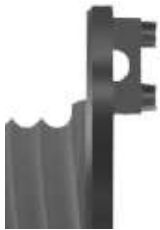
Rope clamp outside of flange
